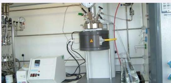
*Pressurised reactor to conduct the acid hydrolysis*
