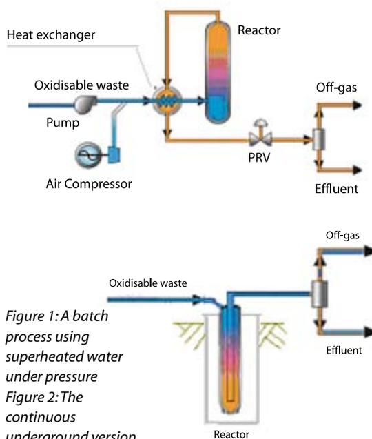
Figure 1: A batch process using superheated water under pressure
